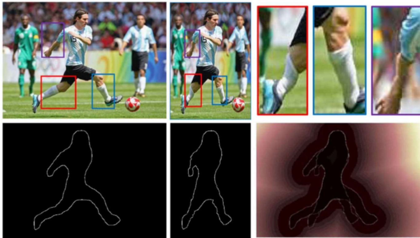
Fig. 3. Local and global shape twisting in image retargeting. Top row shows the original image, retargeted image and several shape twisting areas. Bottom row shows the original and retargeted shape contours of one instance ‘person,’ together with the Chamfer distance map ( DM ).
