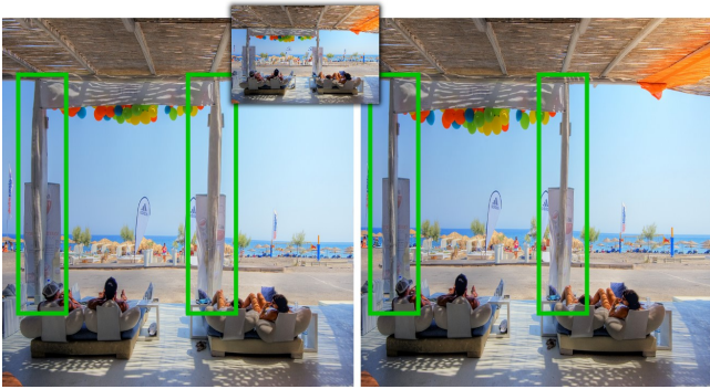
Figure 6: The original image (inset) is expanded in height. The sky region is stretched to reduce distortion, causing the quads covering various regions of the pillars to be scaled to different sizes (left). We solve an optimization problem to make the sizes of connected prominent quads similar; this keeps the uniform thickness of the pillars (right).
