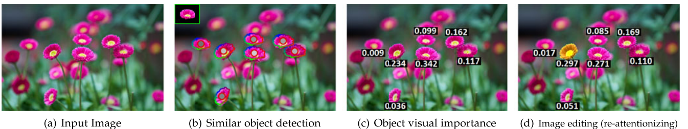
Fig. 2. After detecting and segmenting the similar objects from an input image, we can predict the visual importance of each object. This information can be used in several object-based image editing applications. The numbers on the objects represent the importance value.
