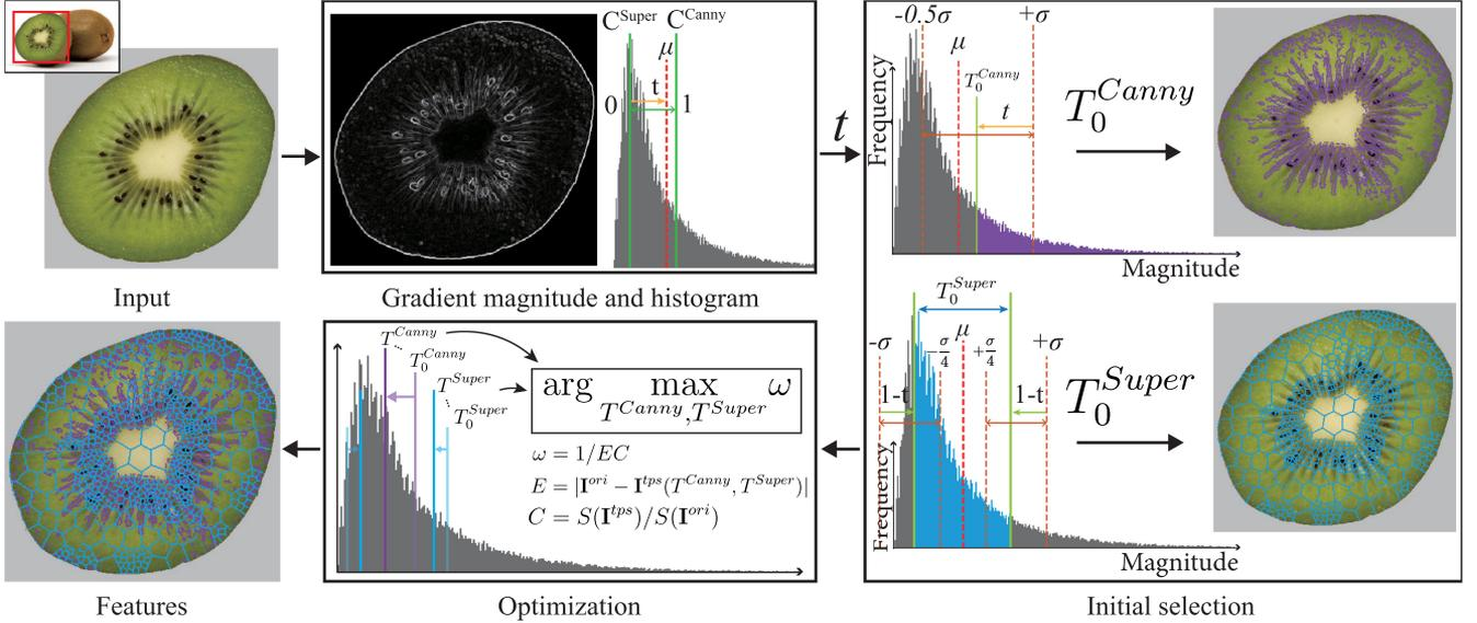
Fig. 7. Selection process of optimal features involving computation of pixel intensity gradients and their corresponding gradient histograms, selecting an initial set of parameters,  $(T_0^{Canny}, T_0^{Super})$ , and determining the final values of  $(T^{Canny}, T^{Super})$  with Monte Carlo searching [30].
