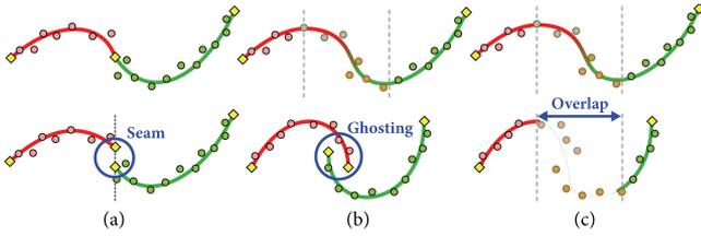
Fig. 11. We simplify TPS interpolation with simplified 2D spline fitting and interpolation using independent fitting and manipulation (a), correlation fitting and independent manipulation (b), and correlation fitting and manipulation (c) where the dots with solid red color are features for the left segment and the dots with green ring are for the right.
