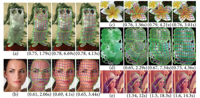
Fig. 4. Parametric patches created using various labeling maps: (a) to (e) Buddha, Face, Flower, Green jade, and Lena. The first column is the original raster image, and second to fourth columns are parametric structures created using different labeling maps along with their corresponding reconstruction mean square error and GPU-based TPS run times.
