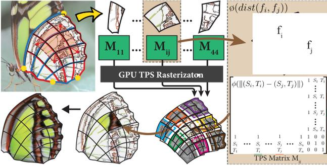
Fig. 10. Our localized patch TPS scheme consists of patch decomposition, equal-number feature patch extension, TPS kernel formation, TPS kernel inversion, rasterization, and overlapping interpolation.
