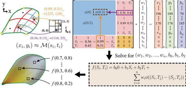
Fig. 8. Our TPS matrix construction consists of transforming the feature locations from pixel coordinate to parametric coordinate and filling  $\mathbf{K}$ ,  $\mathbf{P}$ , and  $\mathbf{W}$  with features' inter-relationship. After inversion, our system rasterizes the  $i$ -th pixel by transforming to parametric coordinate and estimating its color using  $f(S_i, T_i)$  listed in Eq. (3).
