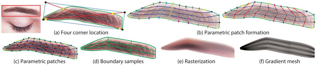
Fig. 3. A parametric patch is constructed by identifying four corners: (a) computing the location and derivatives of  $M \times N$  control points; (b) create the Hermite patch  $\mathcal{M}(s, t)$ ; (c) sample detailed features at patch boundaries; (d) and rasterize the results. (e) We also constructed a faithful gradient mesh of very dense primitives (f).
