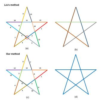
Fig. 12. (a), (c) The different colors of line segments denote the number of line segments to be connected and the numbers on the figure denote the connecting sequence. (b) The result of Liu's method using five different wires (i.e., with five different colors) to connect a star. (d) The result of our method using one wire to connect a star, i.e., needs a single blue color wire.
