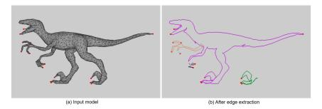
Fig. 7. The result without the constraint (3). The extracted edges are disconnected.
