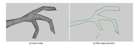
Fig. 9. Without this constraint (4), the extracted edges can be disconnected.
