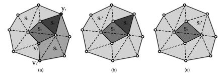
Fig. 8. The merging of  $S_3$  and  $S_4$  with shared vertex  $V_b$  not on the merged edge. This could also separate the extracted edges. (a)  $V_1$ ,  $V_2$ , and  $V_b$  are all the merged vertices between  $S_3$  and  $S_4$ . (b) The result of merging  $S_3$  and  $S_4$ .  $S_3$  is the merged set. (c) After merging of  $S_2$  and  $S_3$ .  $S_2$  is the merged set.
