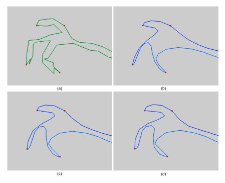
Fig. 17. The comparison of the results with different  $\alpha$  values. (a) Rough wire. (b) Smoothed wire with  $\alpha=0.5$ . (c) Smoothed wire with  $\alpha=1.0$ . (d) Smoothed wire with  $\alpha=2.0$ .
