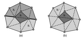
Fig. 6. The combination of  $S_2$  and  $S_3$  with discontinuous shared edges. This will separate the extracted edges. (a) The shared edges between  $S_2$  and  $S_3$  are not continuous. (b)  $S_2'$  is the combined set of  $S_2$  and  $S_3$ .
