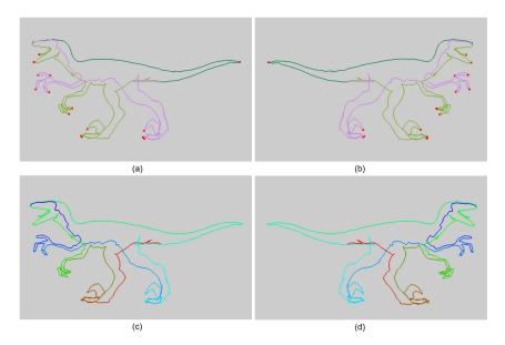
Fig. 14. The result of wire composition. (a) The three edge segments (in different colors) extracted in the previous step. (b) Another view of the edge segments. (c) After wire composition, only a single continuously rough wire is obtained. We use the red-green-blue gradient color to represent the detour of the wire. (d) Another viewpoint of the rough wire.
