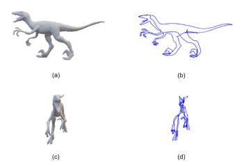
Fig. 20. Comparison between original model and our wire results. Distance error D(a, b) = 0.000236924 and D(c, d) = 0.00131612. Note we will define distance error in Equation (13) later.
