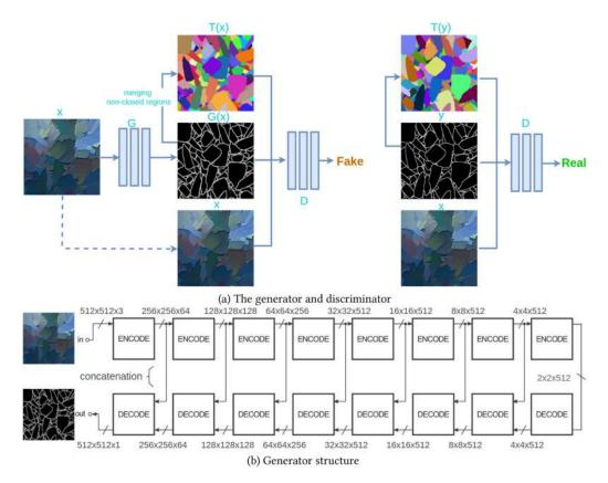
Fig. 7. The modified Pix2Pix network structure. Note that the colors in T(x) and T(y) are used for visualization, but not labels. T(.) denotes edge map that is involved in Pix2Pix network computation. Note that T(x) and T(y) should be of binary image edge maps without colors. Herein we color regions in order to visualize the regions closed.
