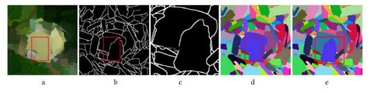
Fig. 6. An example of blurred edges and gaps within strokes. (b) Edge map by Pix2Pix from (a) input image. (c) A small gap from (b). (d) Wrongly merging the adjacent regions due to a gap on their boundaries. (e) Correct segmentation.
